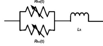
Figure 1: Simple structure of a resistive SFCL
