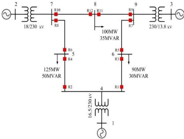
Figure 2: WSCC 3-machine, 9-bus system
