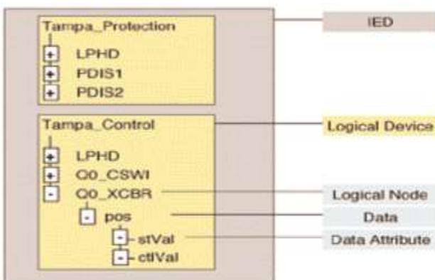
Figure 4: Vertical data model in object-oriented method
