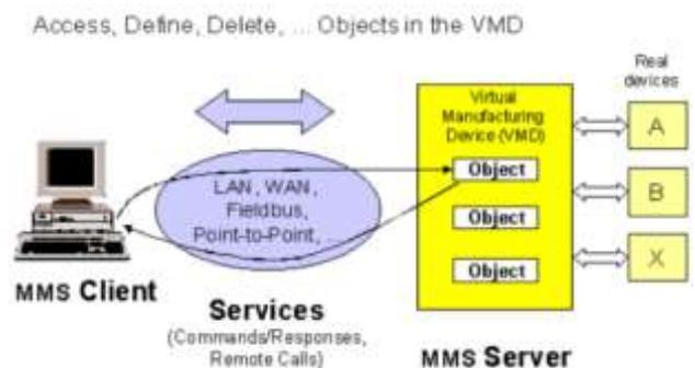
Figure 5: Client model - MMS server
