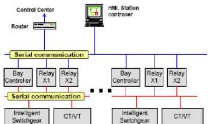
Figure 3: Vertical communication in client-server model [6]
