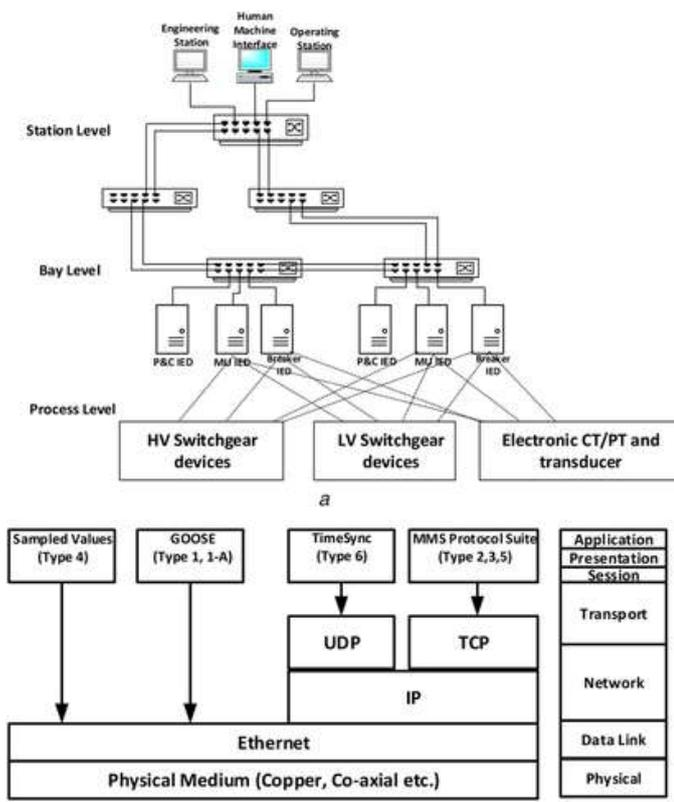
Figure 1: Configuring substation protection using LAN [5]
