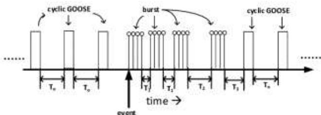
Figure 2: GOOSE message sending intervals with matching capability [5]
